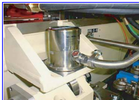
Figure 9b: Level sensor (LS) mounted on the girder. Below it an eccentric cam disc is visible.
