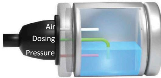
Figure 5. Measuring probe with symbolically drawn connections for pressure, dosing and air compensation. The probe does not contain any electronics and is therefore insensitive to overvoltage.
