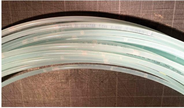
Figure 6. Liquid tube 2 days after first filling. Many bubbles were formed in the liquid during 2 days.
