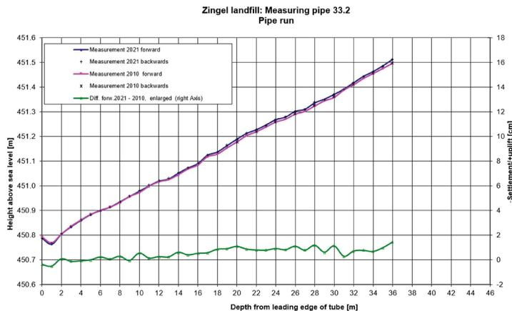
Figure 10. Measurement results from inclinometer tube 33.2, red line: forward and backward measurement 2010, blue line 2021, green line: difference of the two measurements, right scale.
