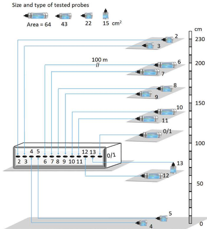
Figure 7. Test setup in the laboratory with probe levels from 0 cm to plus 230 cm.
