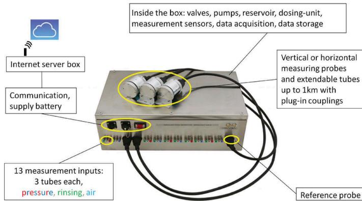
Figure 3. GRIMONIT central unit with two measuring probes and the reference sample connected.
