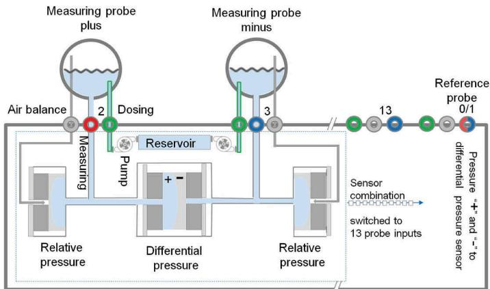
Figure 4. Measuring principle of GRIMONIT: The differential pressure of 2 measuring probes and the relative pressures of each probe are continuously recorded. This combination is switched sequentially to the other measuring inputs with valves. The liquid level in the measuring probes is controlled via the dosing line.
