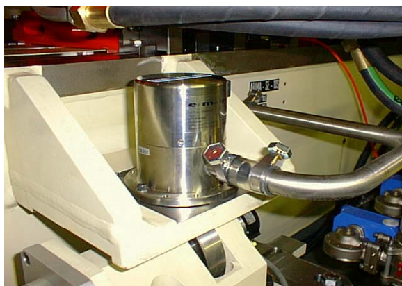
Fig. 5: Level sensor (LS) mounted on the girder. Below it an eccentric cam disc is visible.
